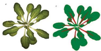
Images taken with VIS camera. Captured image extracted from background (left); color classified (analyzed) image (right).
